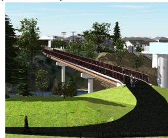
A steel truss bridge was considered because it is a common bridge type in Oregon. The total project cost is estimated to be \$5.0 million in today's dollars, which is second lowest amongst the alternatives. The bridge would be harder to permit because of the columns in the river.
